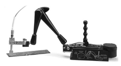
The tip of the Agilent TDR Probe incorporates a novel variable pitch, spring-loaded ground pin. The spring-loaded feature enables compensation of different height ground and signal contacts. This will easily accommodate manufacturing tolerances of standard printed circuit board probing pads.
